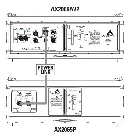
The module employed for powering the AX2065AV2 delivers in an ultra-compact package a maximum power of 2800W. Moreover, each AX2065AV2 is able to power an additional passive AX2065P module through the available power output on the back panel. This feature will allow to assemble very competitive system solutions both for rental and installation applications.
